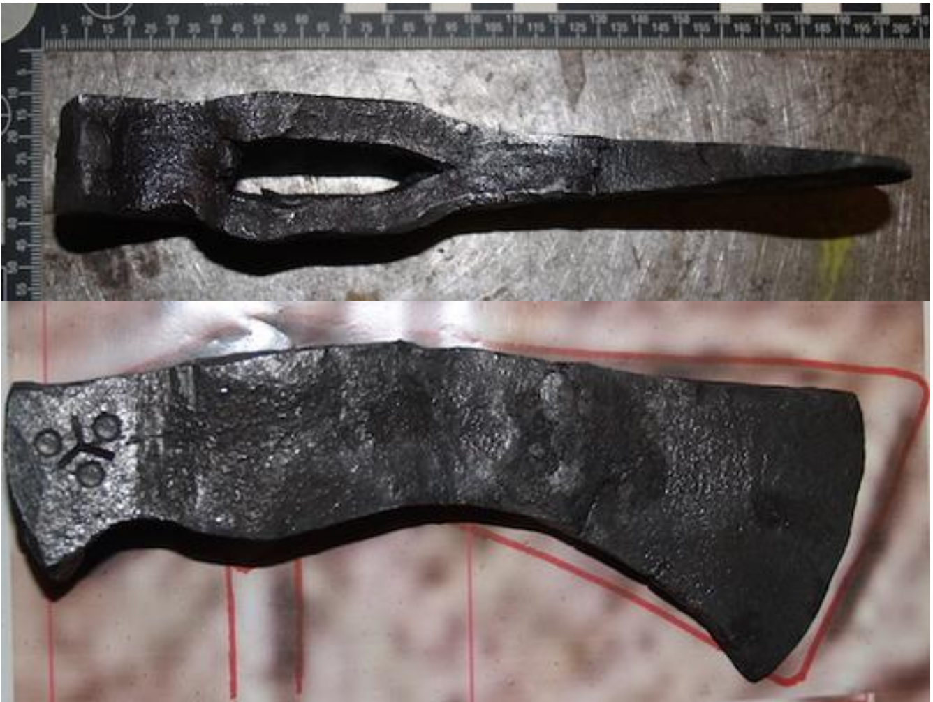
Figures 19 & 20: Completed bloomery iron replica, top and right side view (with maker's mark)
