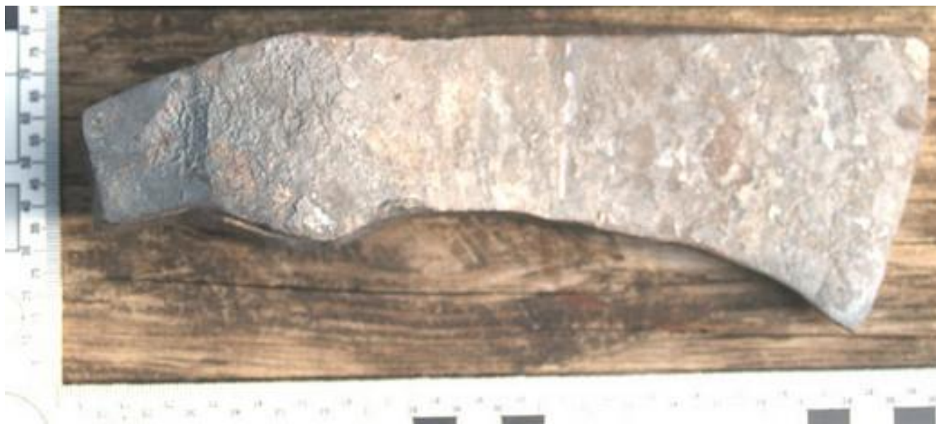
Figure 15 : Prototype of the Axe – about life sized Rough forged weight = 1005 gm
