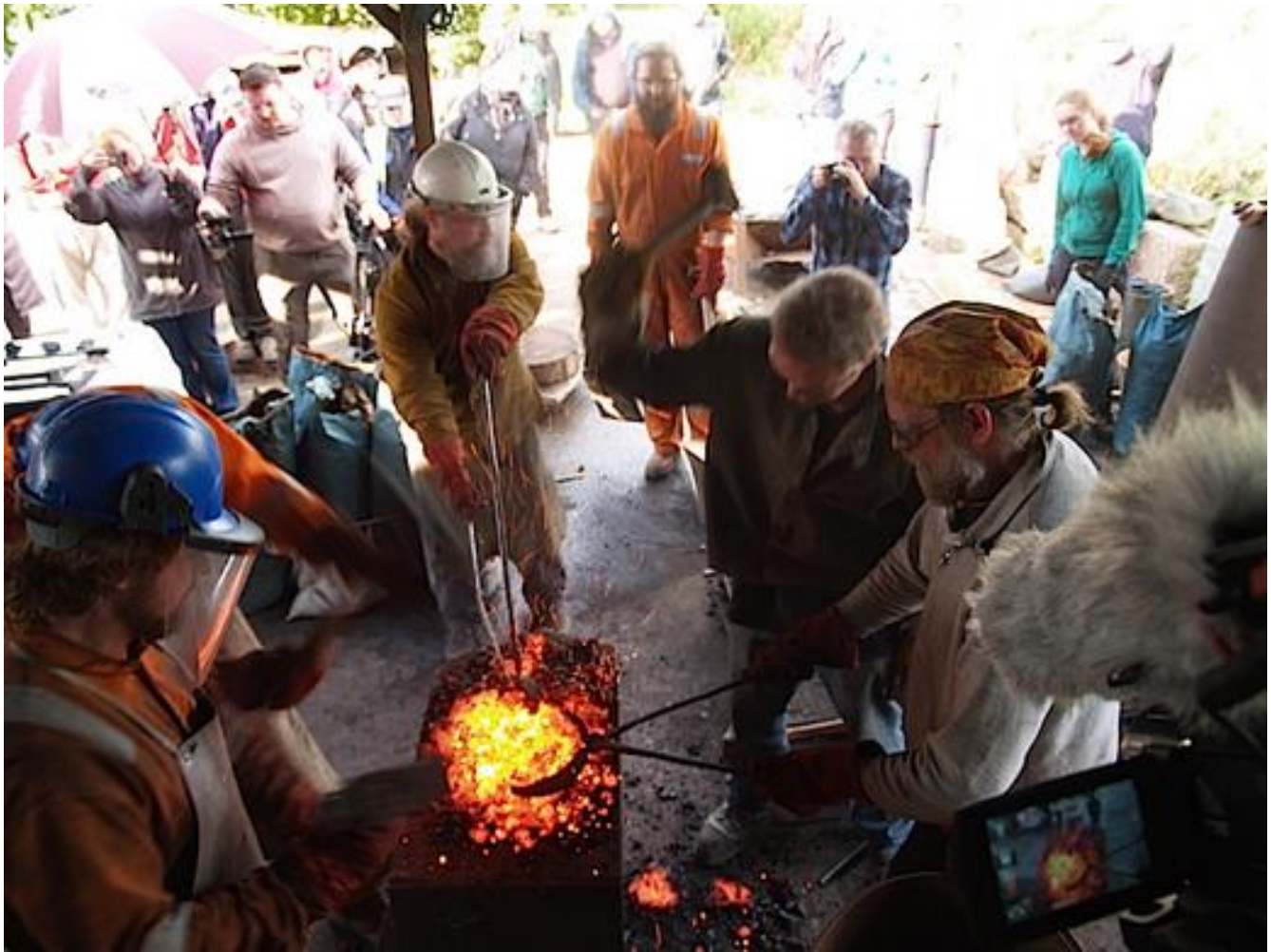
Figure 21 : Bloom consolidation before the public, smelt 1.3.
